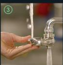
1) The downward orientation of the eyePOD eyewash nozzles, when not in use, keeps them free of dust and debris accumulation, and allows your faucet to function normally. 2 & 3 Rotating the front of the eyePOD one-half turn (in either direction) brings the eyewash spouts to the top and automatically resets the unit to operate as an eyewash.
